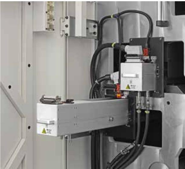
H-UV L(LED) lamps housed in pullout drawers, making lamp replacement easy.
