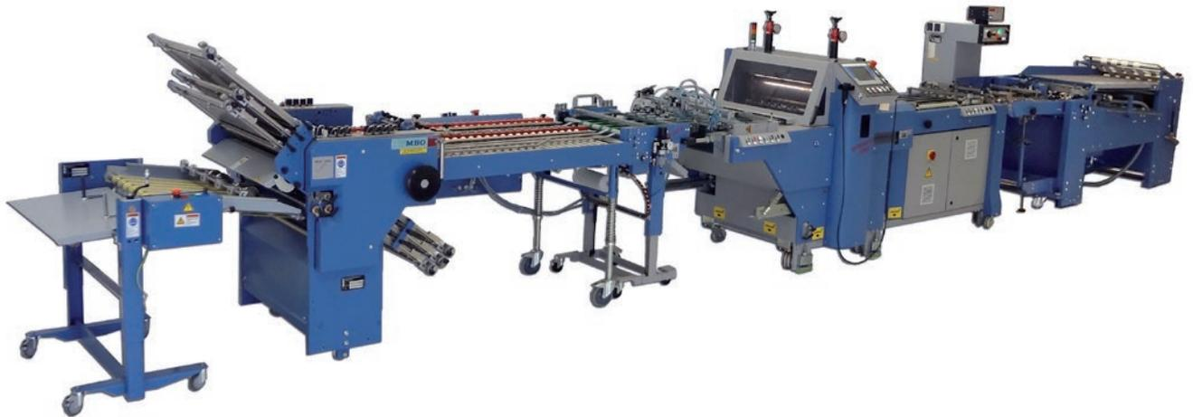
Production line consisting of upstream continuous feeder, BSR 550 Servo, UEB 550 B and downstream buckle plate folder.
