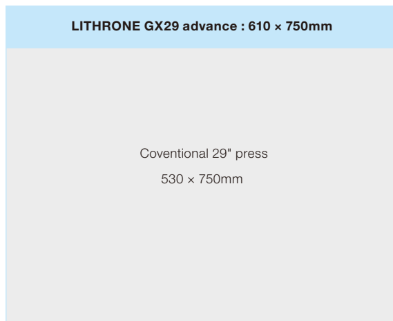
Comparison of standard 29" sheet size vs. Lithrone GX29 advance's maximum sheet size
