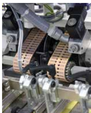
Some of the standard features of the K8RS, from left to right: Palletized feeder, feeder head VacuJet RS, double vacubelt and timing belt drive in the parallel fold.
