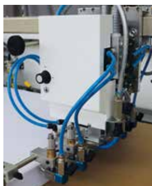
Some of the standard features of the K8RS, from left to right: Palletized feeder, feeder head VacuJet RS, double vacubelt and timing belt drive in the parallel fold.
