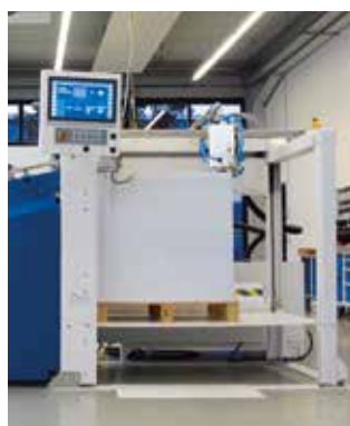
Some of the standard features of the K8RS, from left to right: Palletized feeder, feeder head VacuJet RS, double vacubelt and timing belt drive in the parallel fold.
